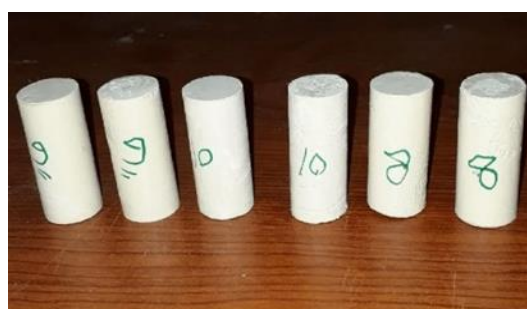
Figure 1. Geopolymer cement paste specimen
