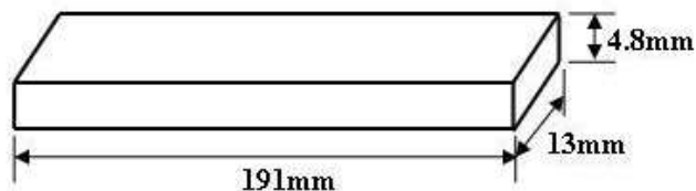
Figure 3 A sketch of bending resistance sample.
