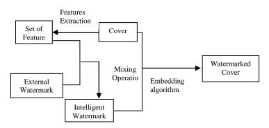
Fig. 1 Embedding watermark Operation
