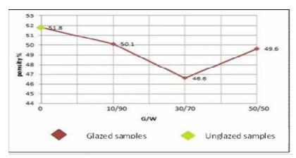
Fig.(1-3):Porosity of A5-glazed samples as a function of G/W mixing
