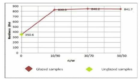
Fig.(1-12): Vickers hardness of A5-glazed samples as a function of G/W mixing ratio
