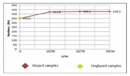
Fig.(1-11): Vickers hardness of A<sub>4</sub>-glazed samples as a function of G/W
