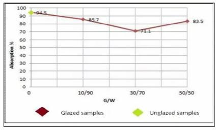
Fig.(1-4):Water absorption of A4-glazed samples as a function of G/W mixing ratio
