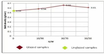
Fig.(1-6): Bulk density of A<sub>4</sub>-glazed samples as a function of
