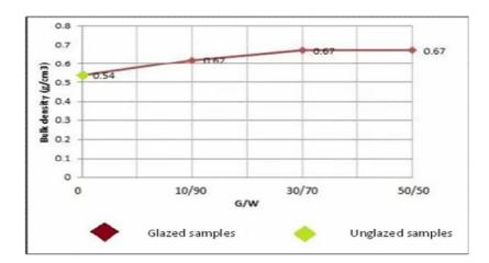
Fig.(1-7): Bulk density of  $A_5$  – glazed samples as a function of G/W
