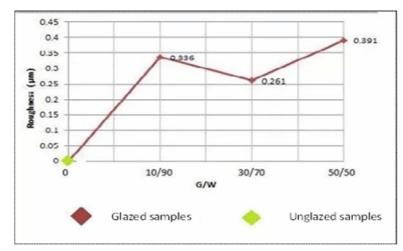
Fig.(1-8): Surface roughness of  $A_5$ -glazed samples as a function of G/W mixing ratio
