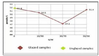
Fig.(1-2):Porosity of A<sub>4</sub>-glazed samples as a function of G/W
