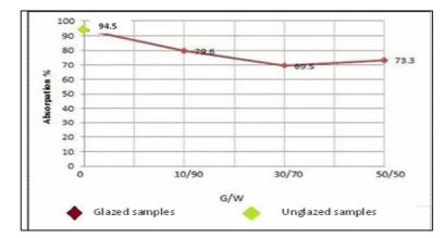
Fig.(1-5): Water absorption of A5-glazed samples as a function of G/W
