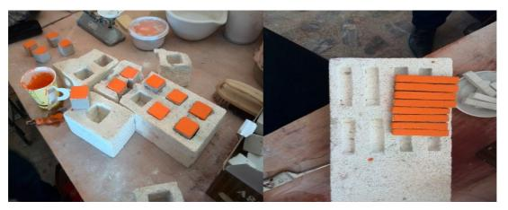
Fig(1-1): Cubic holes in the fire bricks
