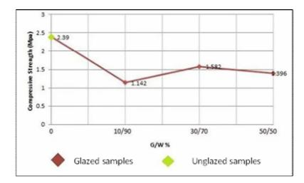
Fig.(1-9): compressive strength of A<sub>4</sub>-glazed samples as a function of G/W
