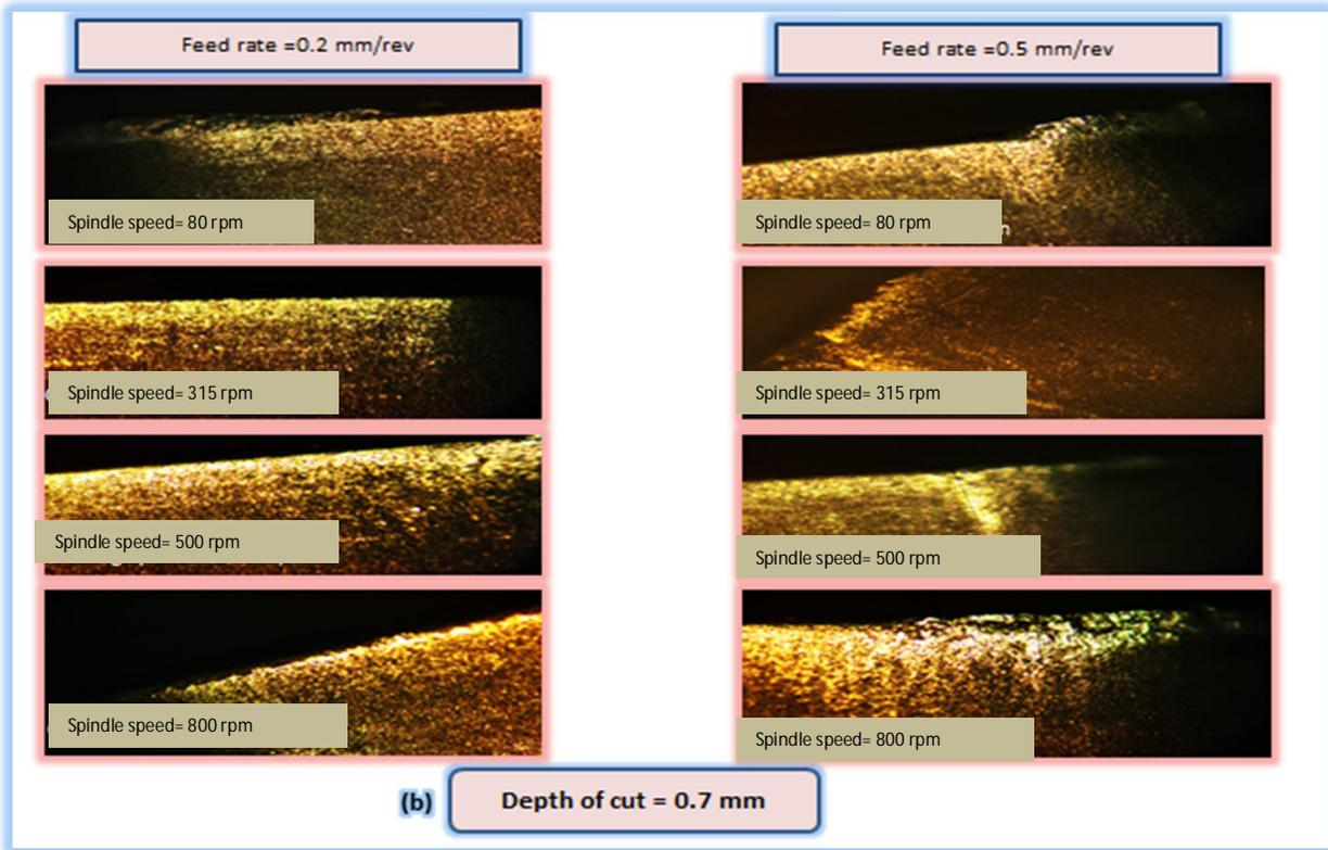
**Figure (3) : The flank wear of the tools during the machining process.**
