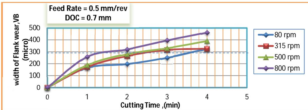
Figure(2): Estimation of the tool life.
