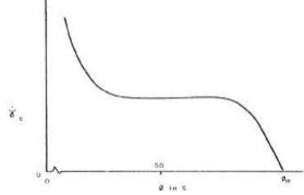
Figure 4: Critical shear rate onset dependence on the volume fraction[9].
