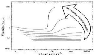
Figure 3: Shear rate/Viscosity curve as a function of different volume fraction[8].
