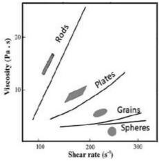
Figure 7: The effect of different shape of particles on the viscosity/shear rate behavior[14] and [4]. E. Attractive forces between particles: The attraction between particles has an important effect to obtain the required rheological properties, as the forces must be stable between particles. To get shear thickening there should be no attraction between the particles as shown by figure 8 [11].
