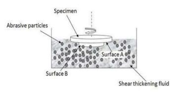
Figure 10: Shear thickening fluid and SiC particles for polishing and cleaning[17].
