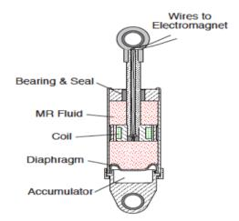
Figure 9: Shock absorber system for automotive[15].
