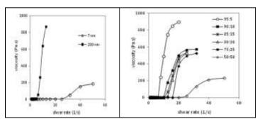
Figure 6: The effect of particle diameter (left) and particle size distribution (right) on the shear thickening behavior [13].
