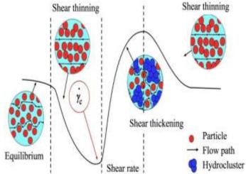
Figure 2: The shear thickening fluid behavior [7].
