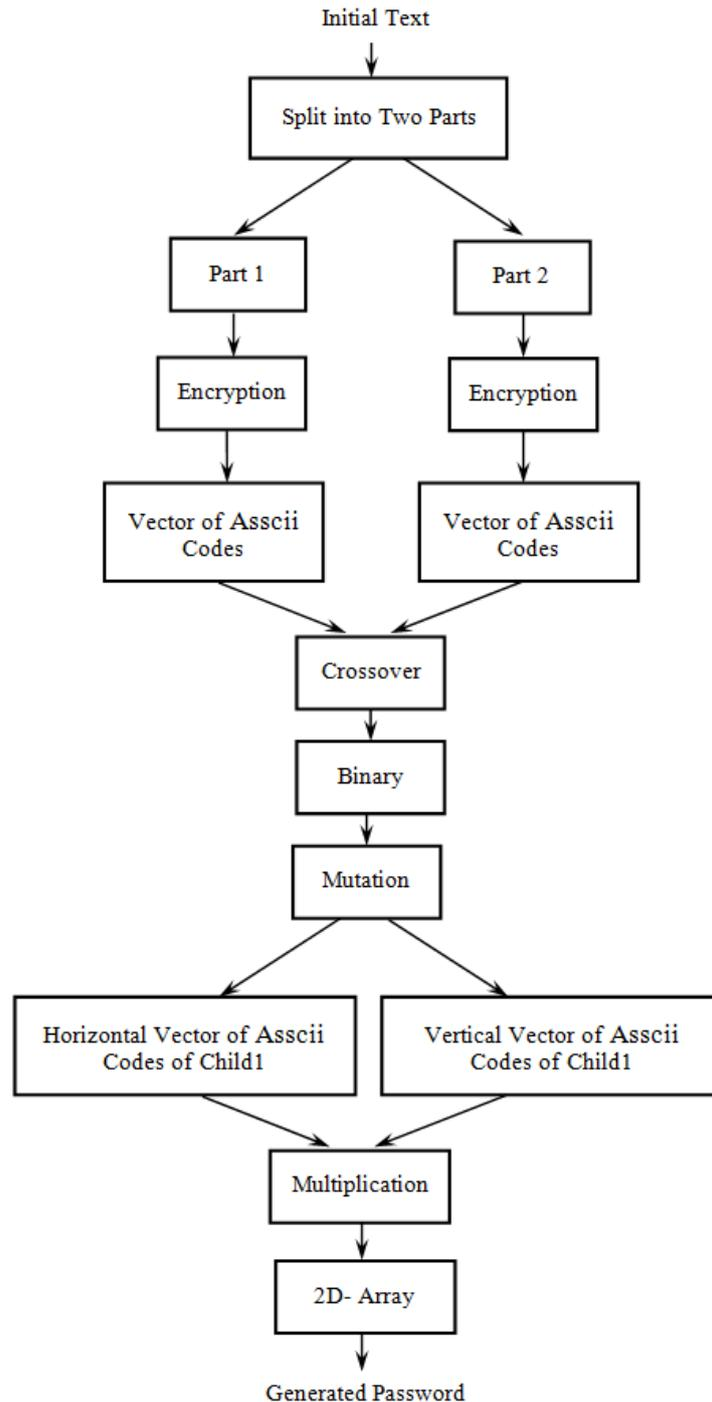
**Figure (1) Text Based Password Generation.**
