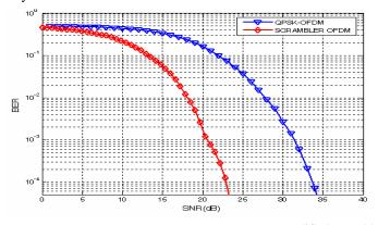
Fig.13. BER performance of scrambler -OFDM using modified scrambler in Flat Fading Channel at Max Doppler Shift=10Hz.
