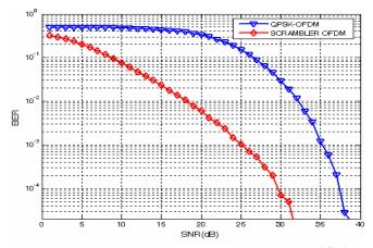
Fig.14. BER performance of scrambler -OFDM using modified scrambler in Selective Fading Channel at Max. Doppler Shift=10Hz.
