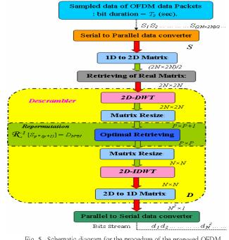
Fig. 5. Schematic diagram for the procedure of the proposed OFDM Receiver
