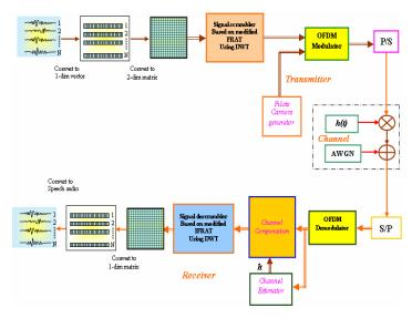
Fig.3. Block Diagram of scrambler OFDM System Based on modified FRAT using DWT
