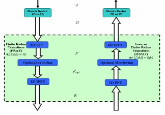
Fig.1. Schematic diagram for the mechanism of the FRAT and IFRAT transform
