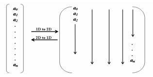
Fig. (2) Graphical illustration of matrix converter operations for both **1D** vector to **2D** matrix & **2D** matrix to **1D** vector
