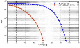
Fig .12. BER performance of scrambler -OFDM using modified scrambler in AWGN channel model
