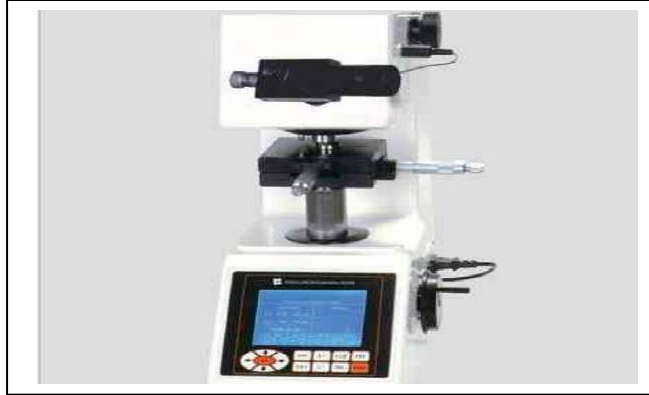
Fig. 5: Vickers microhardness measuring machine (HVS-1000).
