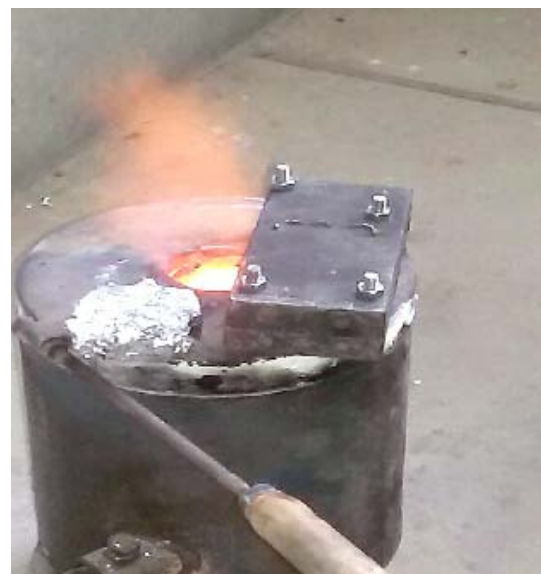
Fig. 2: Gas furnace used for melting
