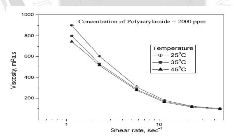
Figure 15: Effect of temperature on viscosity of polymer solution[33].
