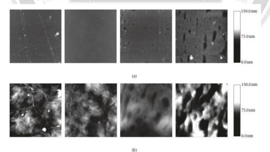
Figure 12: AFM images of PLA, (a) before and (b) after the degradation[29].
