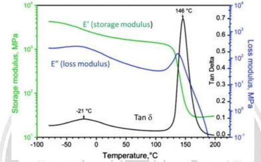
Figure 7: Relationship between E', E'' and tan delta Vs temperature in the DMA[18].
