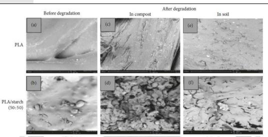
Figure 11: PLA and PLA/starch composite SEM images before and after degradation[29].
