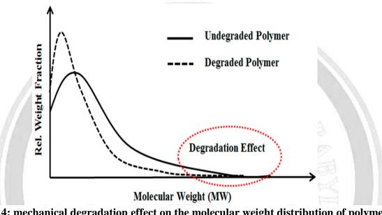
Figure 14: mechanical degradation effect on the molecular weight distribution of polymer
