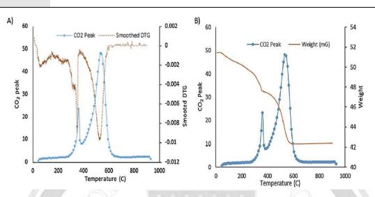
Figure 10: TGA/FTIR analysis of used CLSR catalyst B, A) CO<sub>2</sub> against smoothed DTG B) CO<sub>2</sub> against weight loss of catalyst[25].
