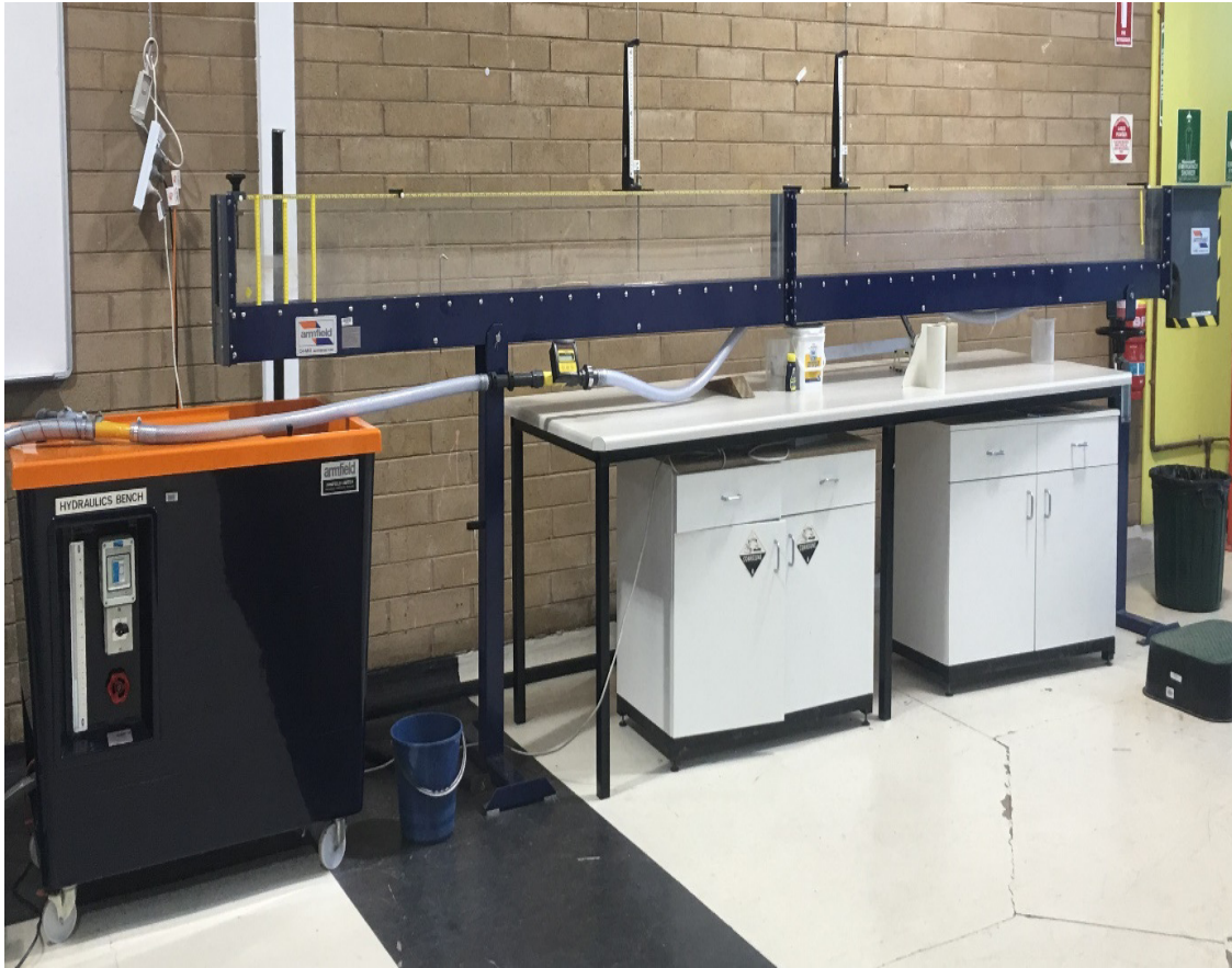
Figure 1B Flume used in experimental work
