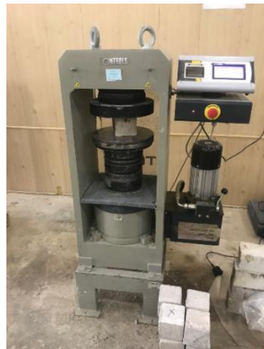
Figure 3: Compression test machine.
