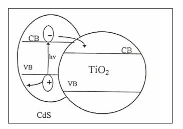
Figure(1):- Illumination of coupled TiO<sub>2</sub>/CdS.
