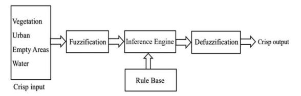
Figure 4. Block diagram of FL system structure.
