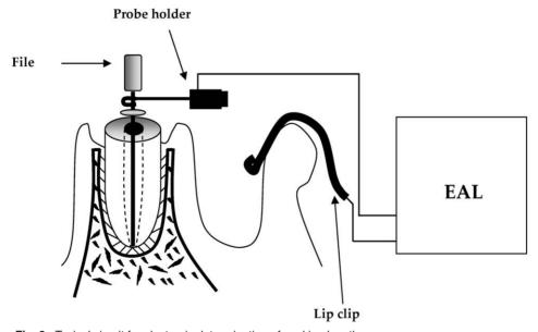
Fig. 3. Typical circuit for electronic determination of working length
