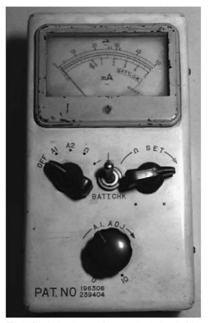
Fig. 2. Simple d.c. ohmmeter for measuring the length of the root canal using direct electric current
