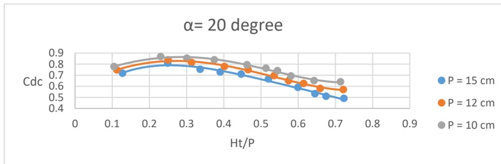
**Figure 7.** Comparison values of  $C_{dc}$  versus  $Ht/P$  for various ( $P$ ) for flat crest trapezoidal labyrinth weir and  $\alpha = 20^\circ$ .
