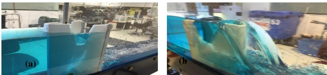
**Figure 5.** Explain nappe interference. (a) before the submerge for  $\alpha^\circ = 21^\circ$ . (b) nearby crest that nappe observe collisions with nappe of other side for  $\alpha^\circ = 16^\circ$ .
