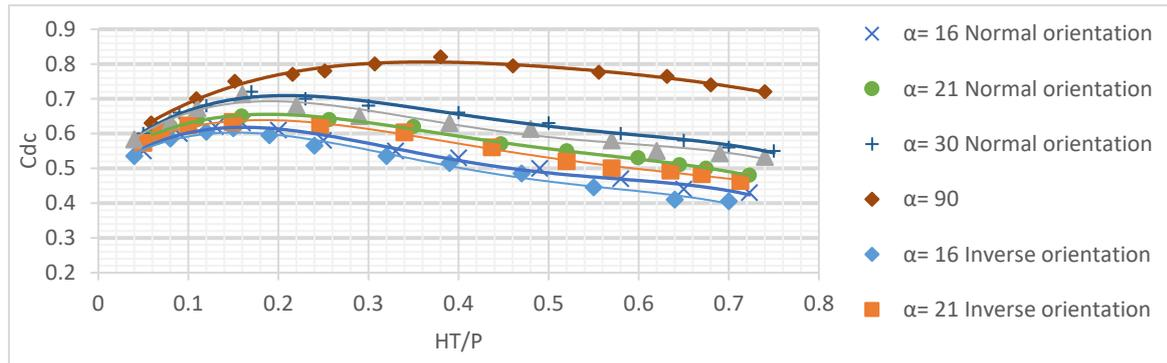
**Figure 6.** Comparison between the normal and inverse orientation of labyrinth weir.
