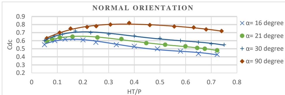
**Figure 3.** The relationship between  $C_{dc}$  values and  $Ht/P$  for flat crest of trapezoidal compound labyrinth weir
