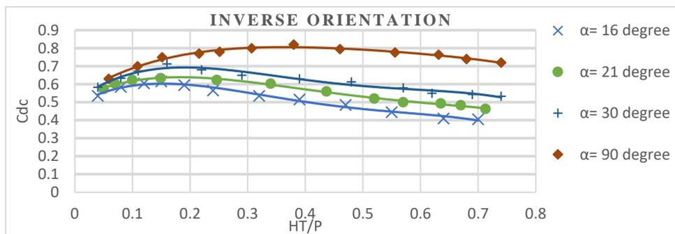
**Figure 4.** The relationship between  $C_{dc}$  values and  $Ht/P$  for flat crest of trapezoidal compound labyrinth weir
