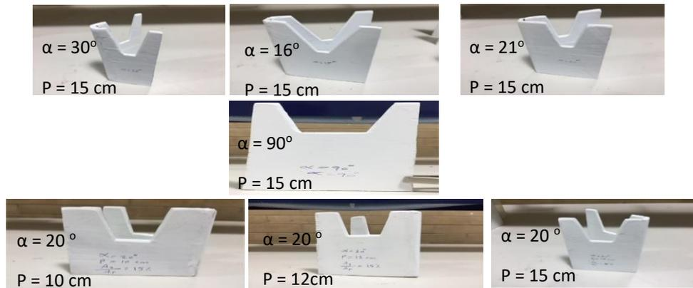
Figure 2. Explain the test models
