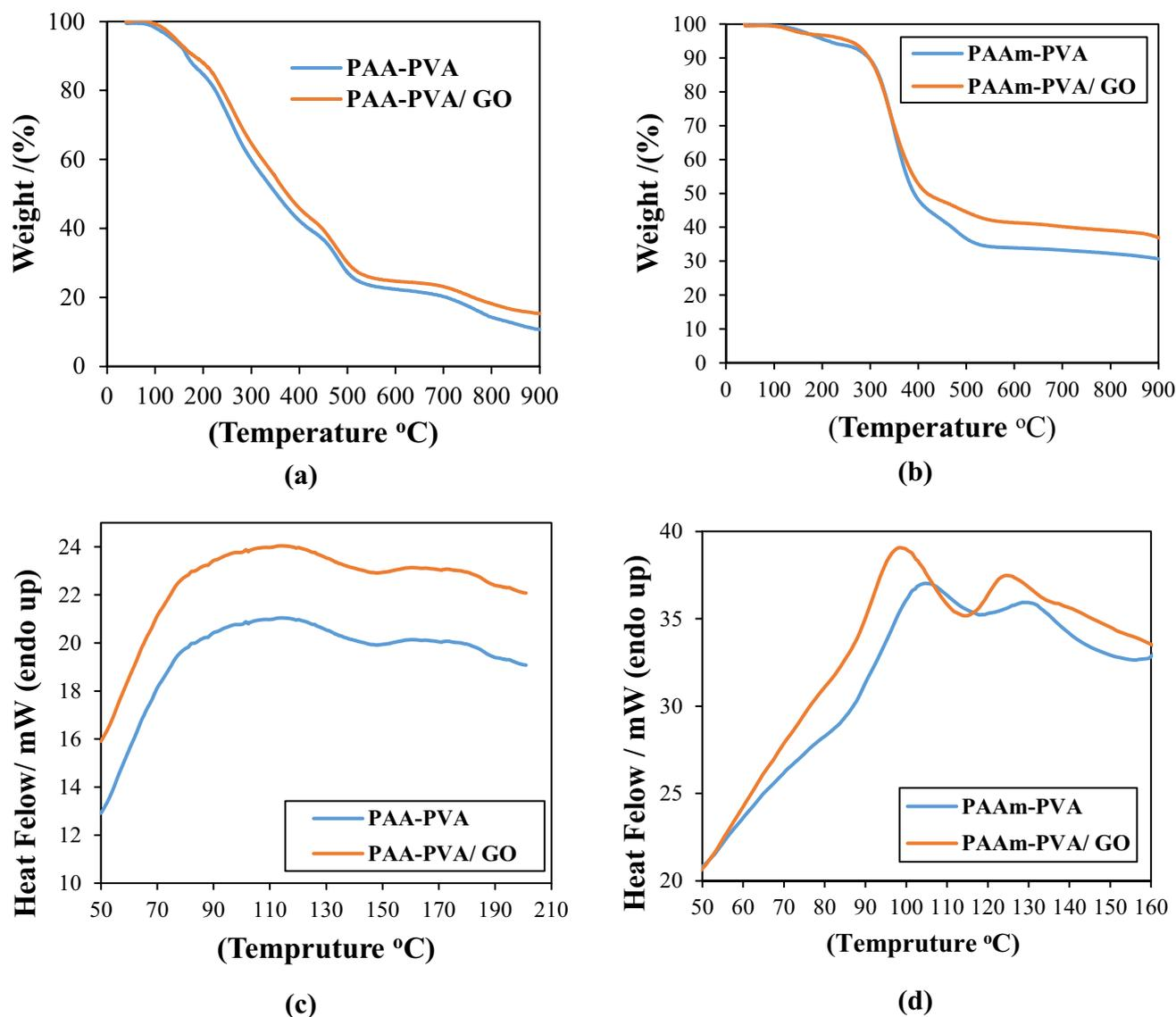
**Fig. 5** (a and b) the thermal gravimetric analysis and (c and d) the differential scanning calorimetry of the samples
