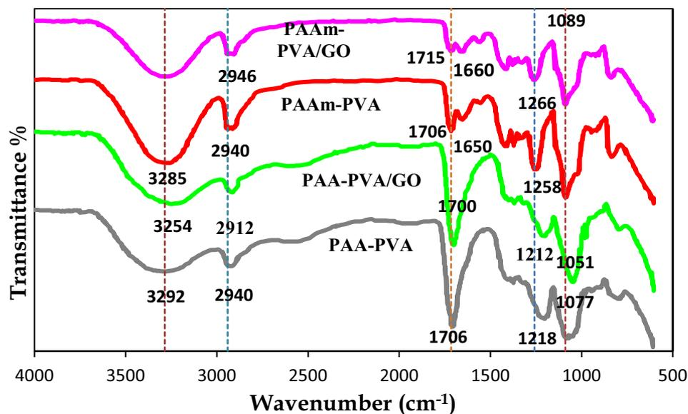
1715 to 1706, 1660 to 1650, and 1266 to 1258  $\text{cm}^{-1}$  of the spectra of PAAm-PVA/GO nanocomposites compared with PAAm-PVA blended polymers, this behaviour agreed with other findings [2, 4, 14].
