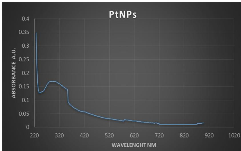
Fig 1: SPR Spectra of PtNPs in DDW
