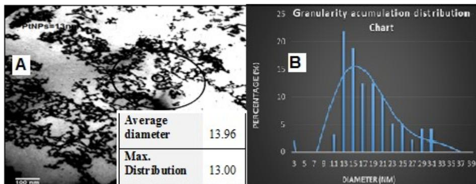
Fig.2: TEM image with  $\times 92000$  magnification power and the granulate accumulation distribution chart for PtNps.
