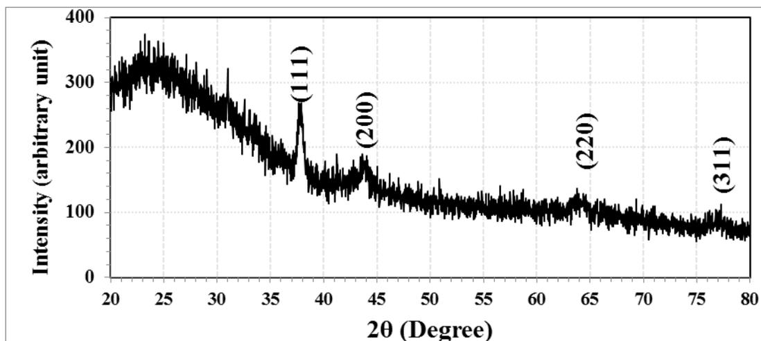
Fig.3: X- Ray diffraction patterns of ptmps prepared by laser ablation technique
