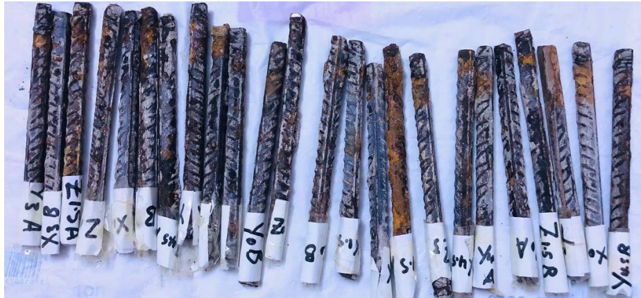
Figure 6: Corroded Steel Reinforcement
