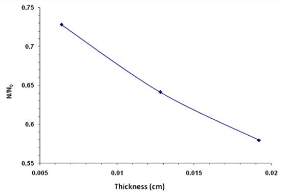
Figure 3.  $N/N_0$  Variation with thickness for 5 wt.% Ti NPs
