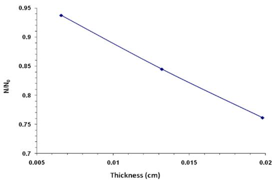
Figure 1.  $N/N_0$  variation with thickness for pure polymer
