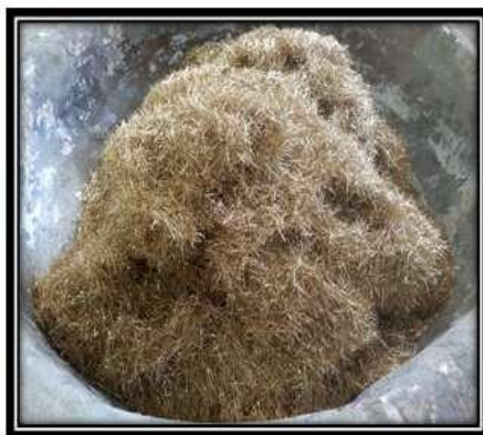
Figure 1 Ultra-Fine Steel fibers
