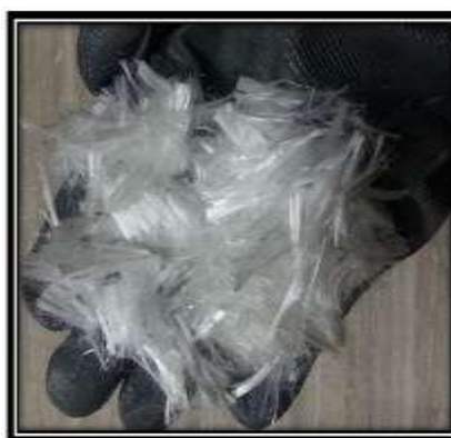
Figure 2 Micro polypropylene fibers
