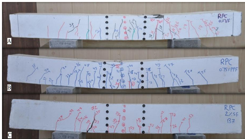
Figure 12 Mode of failures of RPC (A)0% V_f , (B)0.75% PPF and (C)2% SF.
