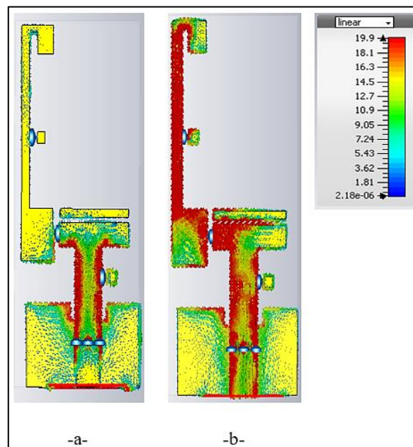
Figure 10. Current distribution of the proposed antenna: (a) ON state at 2.45 GHz resonant freq., (b) OFF state at 5.4 GHz resonant freq.
