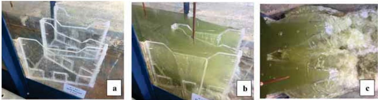
Figure 4. Compound Labyrinth weir with \alpha=15^\circ (a) set up the model inside flume, (b) low discharge over notch, (c) high discharge over entire weir
