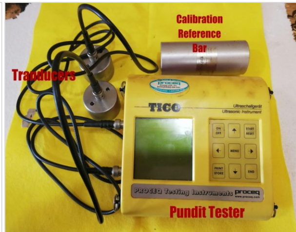
FIGURE 12. Ultrasonic testing of concrete sample.
