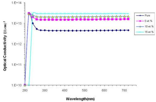
Fig. 9 Optical conductivity of (PVA-PEO-CuO) samples with concentrations of CuO nanoparticles
