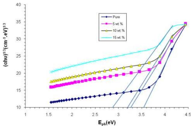
Fig. 4 Energy gap for transitions of forbidden indirect for (PVA-PEO-CuO) nanocomposites
