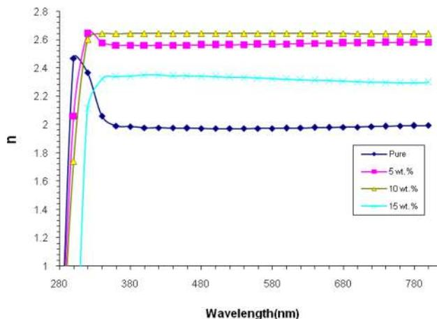
Fig. 6 Refractive index of (PVA-PEO-CuO) nanocomposites as a function of wavelength
