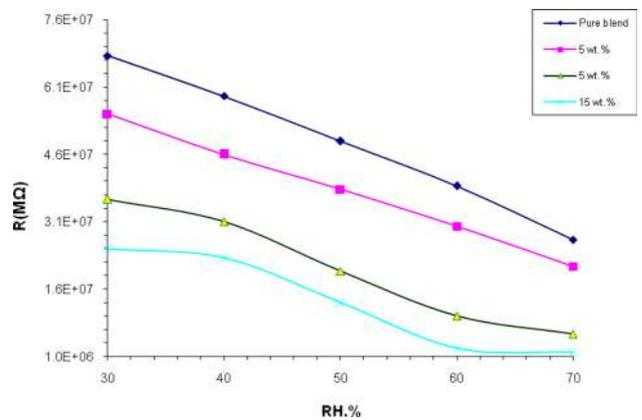
Fig. 10 Variation of resistance for (PVA-PEO-CuO) nanocomposites with humidity
