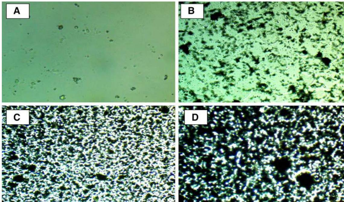
Fig. 2 Microscope images (×10) for (PVA-PEO-CuO) nanocomposites: a for blend b for 5 wt% CuO, c for 10 wt%CuO d for 15 wt%CuO
