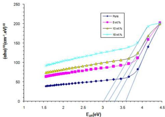
Fig. 3 Energy gap for transitions of allowed indirect for (PVA-PEO-CuO) nanocomposites
