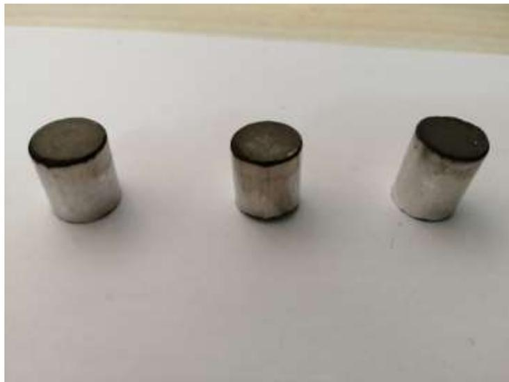
**Figure 1.** (Al/Ni) FGM sample after mixing and pressing.
