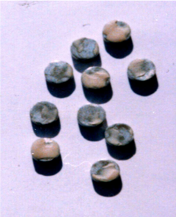
Fig.5: Cohesive failure with remaining porcelain and opaque layers.
