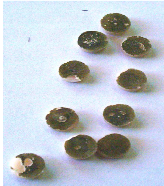
Fig. 4: Dark gray oxide layer on debonded porcelain.
