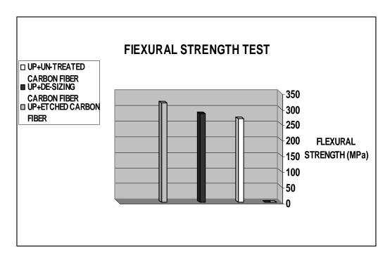
Fig. 2: Flexural strength of unsaturated polyester resin reinforced with and without etched carbon fibers.
