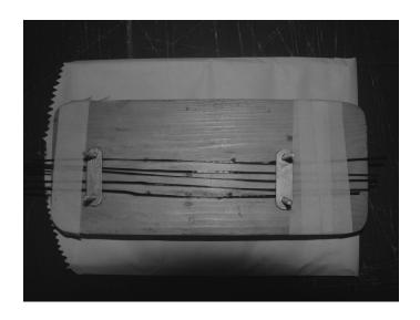
Fig. 1: Flexural sample mold for composite materials
