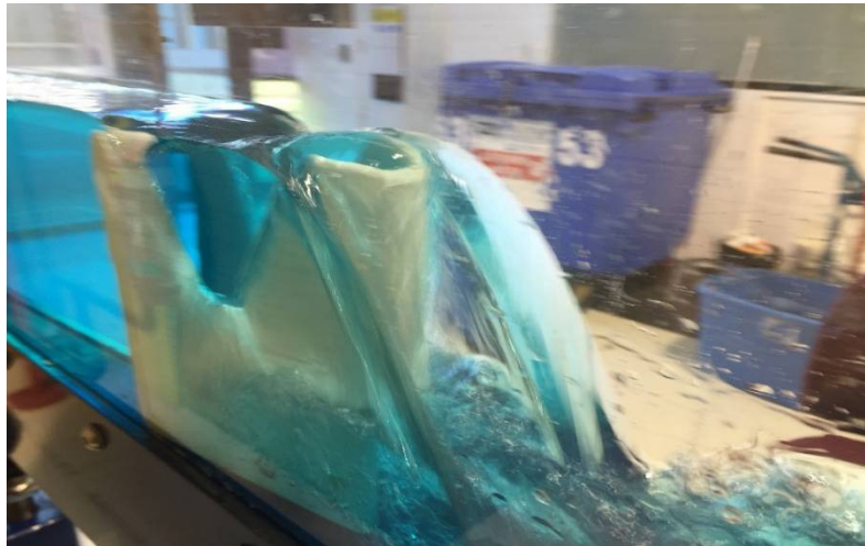
Figure 8 Nappe interference in adjacent crest that observe collisions with each other with \alpha^\circ = 15^\circ .
