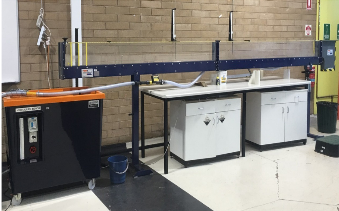
Figure 2 Tilting rectangular laboratory flume at Deakin University civil lab.
