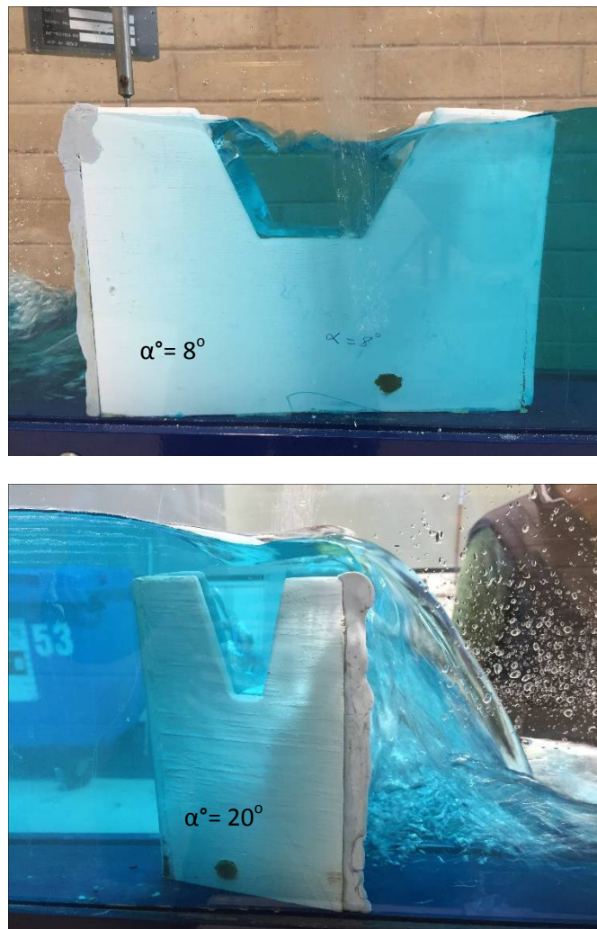
Figure 9 Effect of increasing length of crest on reducing nappe interference, then increasing compound discharge coefficient for \alpha = 8^\circ, \alpha = 20^\circ .
