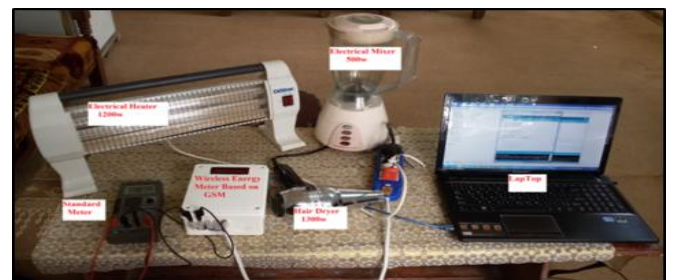
Fig. 18 Loads used with Smart Meter.
