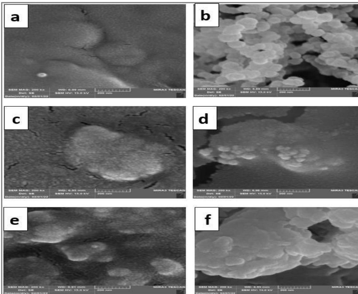
**Fig.2: FESEM for, a. (PVA-PVP) blend, b. (PVA-PVP/ 5wt.% ZnO), c. 1wt.% Ag, d. 2wt.% Ag, e. 3wt.% Ag and f. 4wt.% Ag nanocomposite films.**
