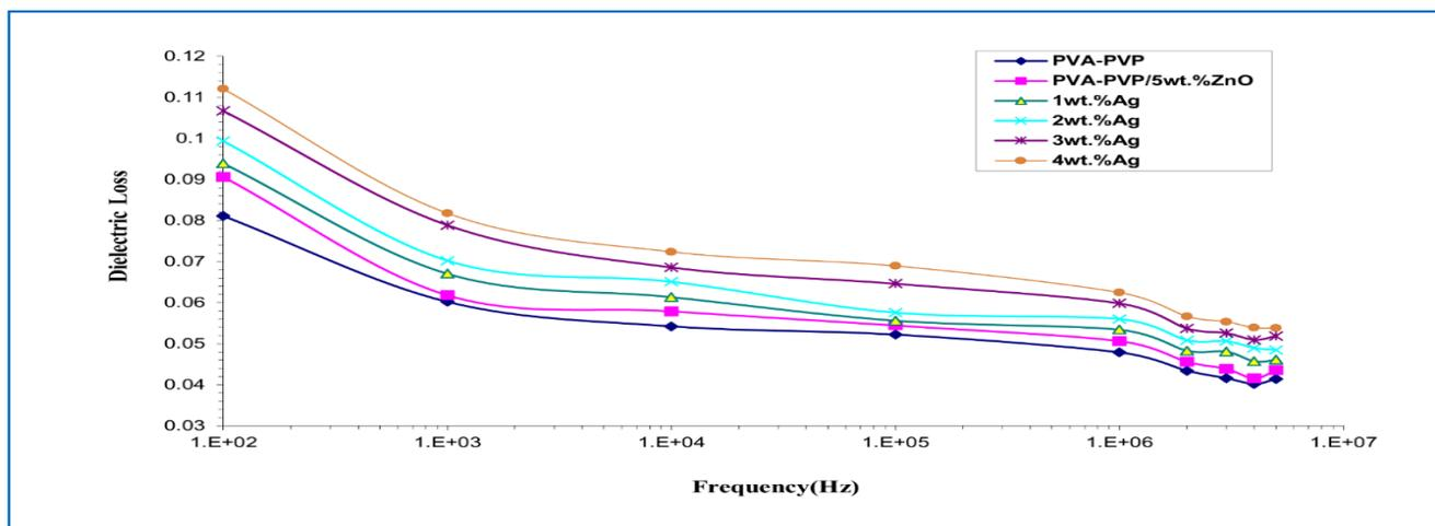
**Fig.4: The dependence of dielectric loss of PVA-PVP blend on frequency and the additives NPs at RT.**
