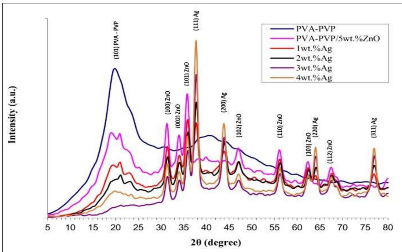
**Fig.1 : XRD patterns of PVA-PVP and it's NCs with ZnO and different wt.% of Ag NPs.**
