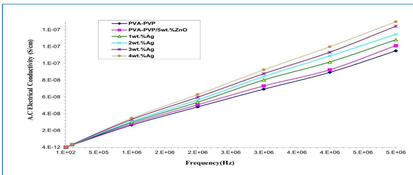
Fig.5: The dependence of A.C electrical conductivity of PVA-PVP blend on frequency and the additives NPs at RT.
