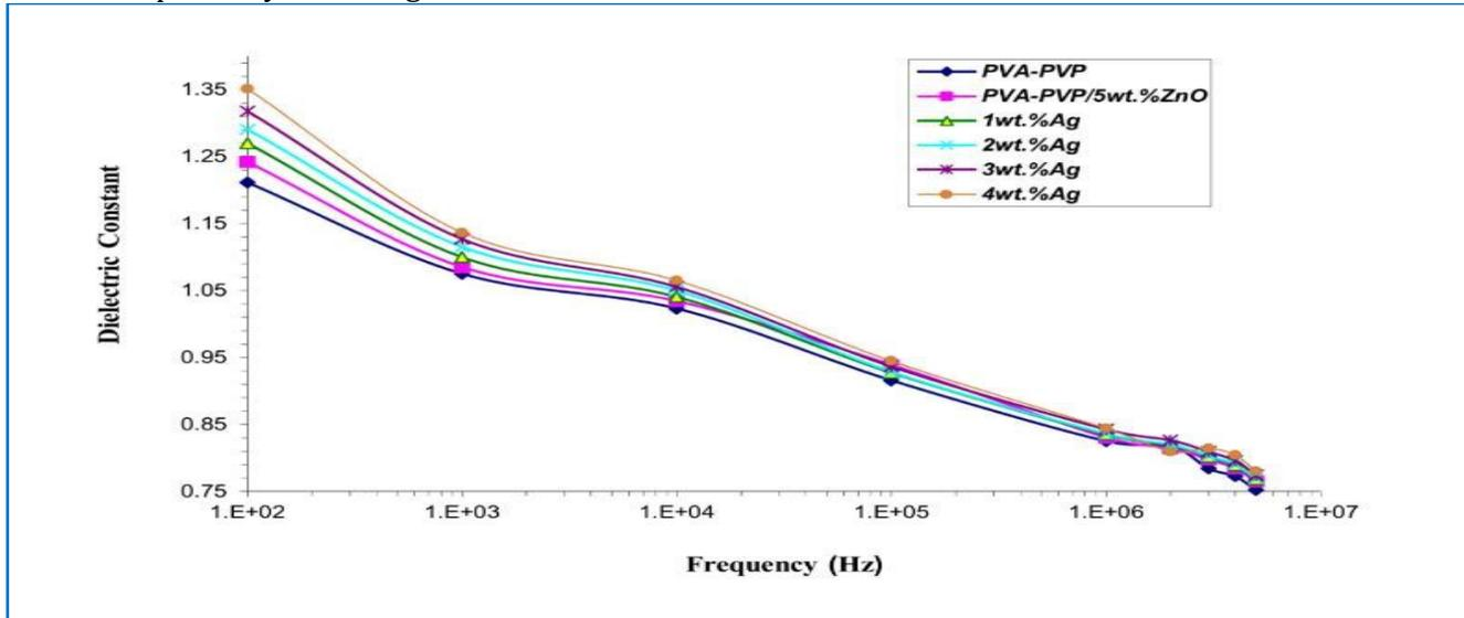
**Fig.3: Dependence of dielectric constant of PVA-PVP on frequency and the additives NPs at RT.**
