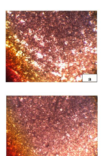
Fig. 4: light optical micrograph for as polished aluminum reinforced by 12wt.%  $\alpha$ -Al<sub>2</sub>O<sub>3</sub> particles (a) before sintering process, (b) after sintering process Alumina particles appear darker than the aluminum matrix.
