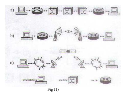
From a mobile or wireless system that has either the source or sink directly at one end of a wireless link [Fig1b], we very likely know some general characteristics of that portion of the link, characteristics that most likely will dominate the TCP tuning algorithms and can therefore be be determined after an initial connection has been established.
