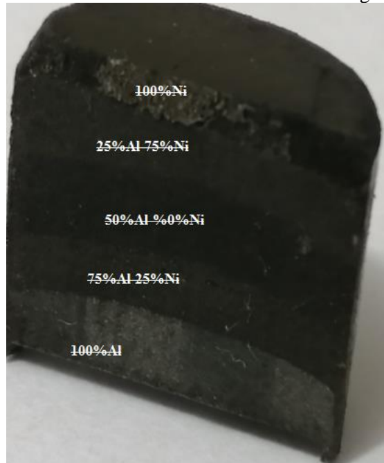
Figure 1. shown the section of a fabricated Al/Ni FGM sample.
