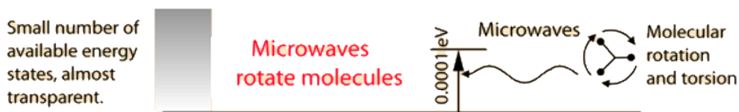
Figure 5: Interaction of microwave radiation with matter
