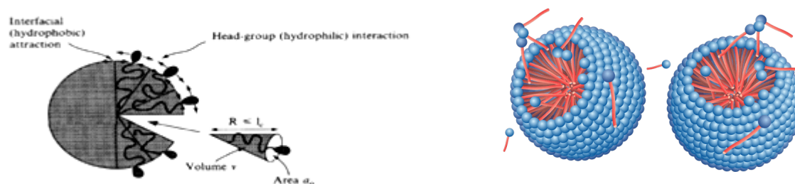
Figure 4 Molecular shapes and critical packing parameter (CPP) of surfactants and lipids and the structures formed (here, v = volume of hydrocarbon core, a_0 = effective head group area, l_c = hydrocarbon chain length).
