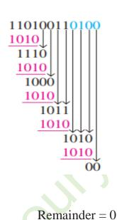
Remainder = 0100. Since the remainder is not 0, append the data with the four remainder bits (blue). Then divide by the generator code (red). The transmitted CRC is 110100110100.
