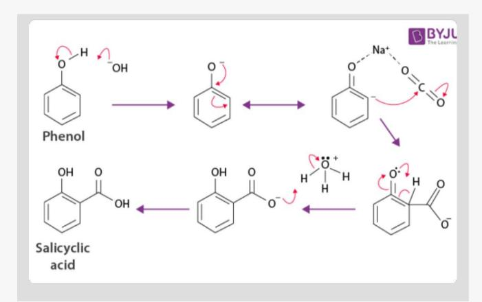
The Kolbe-Schmitt reaction is a carboxylation chemical reaction that proceeds by treating phenol with sodium hydroxide to form sodium phenoxide, then heating sodium phenoxide with carbon dioxide under pressure.
