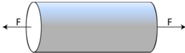
Fig. 3: uniaxial tension \sigma_1 = Y, \sigma_2 = \sigma_3 = 0
