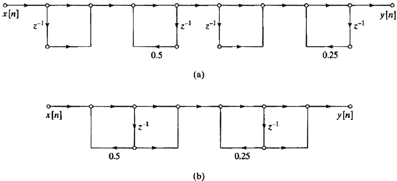
Fig.(1.7): (a) Direct form I subsections.(b) Direct form II subsections.
