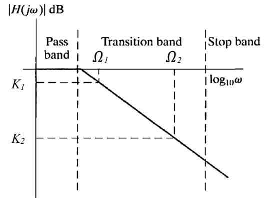
$$\begin{aligned} K_1 &= 20 \log_{10} \frac{1}{\sqrt{1 + \left(\frac{\Omega_1}{\Omega_c}\right)^{2n}}} \\ &= -10 \log_{10} \left( 1 + \left(\frac{\Omega_1}{\Omega_c}\right)^{2n} \right) \end{aligned} \quad (3.3)$$
