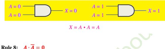
A variable ANDed with its complement is always equal to 0. Either A or A will always be 0; and when a 0 is applied to the input of an AND gate, the output will be 0 also.
