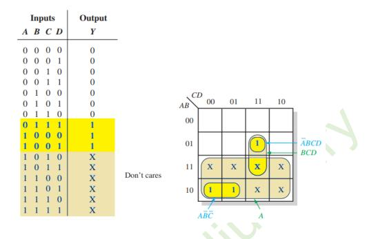
The truth table describes a logic function that has a 1 output only when the BCD code for 7, 8, or 9 is present on the inputs. If the "don't care" are used as 1s, the resulting expression for the function is A + BCD, as indicated in K-map. If the "don't care" is not used as 1s, the resulting expression is ABC + ABCD; so you can see the advantage of using "don't care" terms to get the simplest expression.
