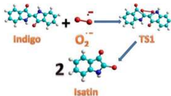
Schem1. The suggested mechanism for the first broken step of indigo dye with \text{O}_2^- .
