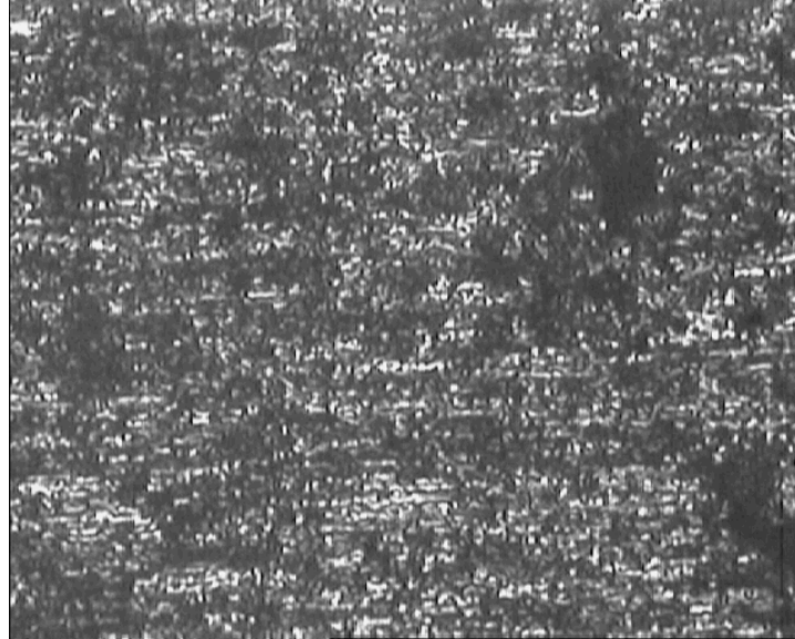
Fig. 3: Light optical microscope image of AMCs reinforced by 10 wt.% SiC (Magnification 400X)
