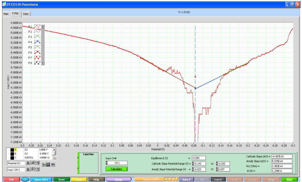
Figure (3) polarization curve of amalgam C in synthetic saliva at 37\pm 1 C°.
