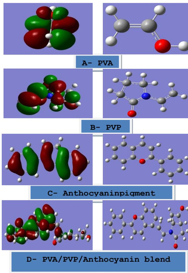
Figure 1: For the considered molecules, (Right): Optimized structures. (Left): HOMO and LUMO shapes.
