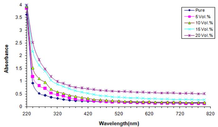
Figure 3: the absorbance versus wavelength for PVA/PVP blend of different adding of anthocyanin volumetric percentages.
