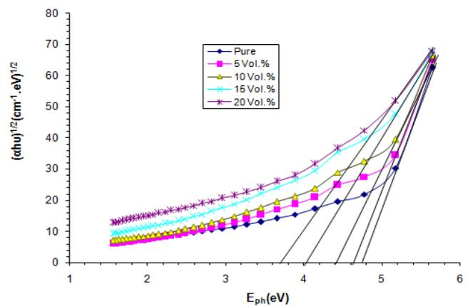
Figure 4: band gap decreasing for PVA/PVP blend with increasing the volumetric percentage of beet juice adding for the allowed direct transition.
