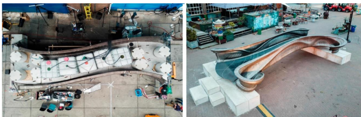
Figure 8: a Load testing of the MX3D bridge; b the MX3D bridge at Dutch Design Week 2018 [61]
