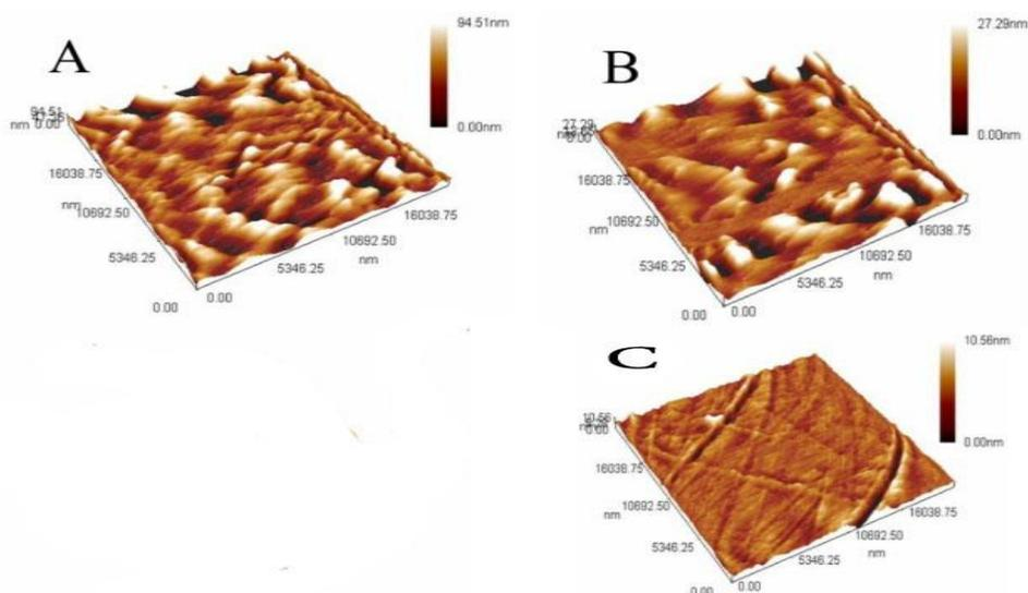
Figure 5. 3D images from AFM of (A) EP pure. (B) 1% ZnO. (C) EP/5% ZnO.
