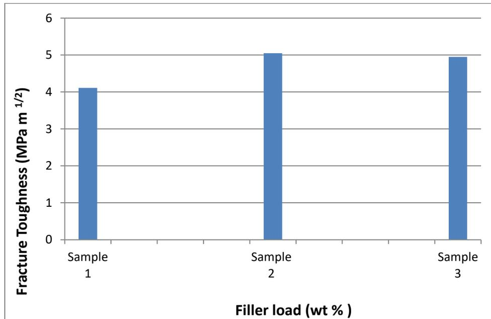
Figure 2. Effect of Fillers Content (wt%) on the Fracture Toughness ( $K_{IC}$ ) of The Epoxy Matrix.
