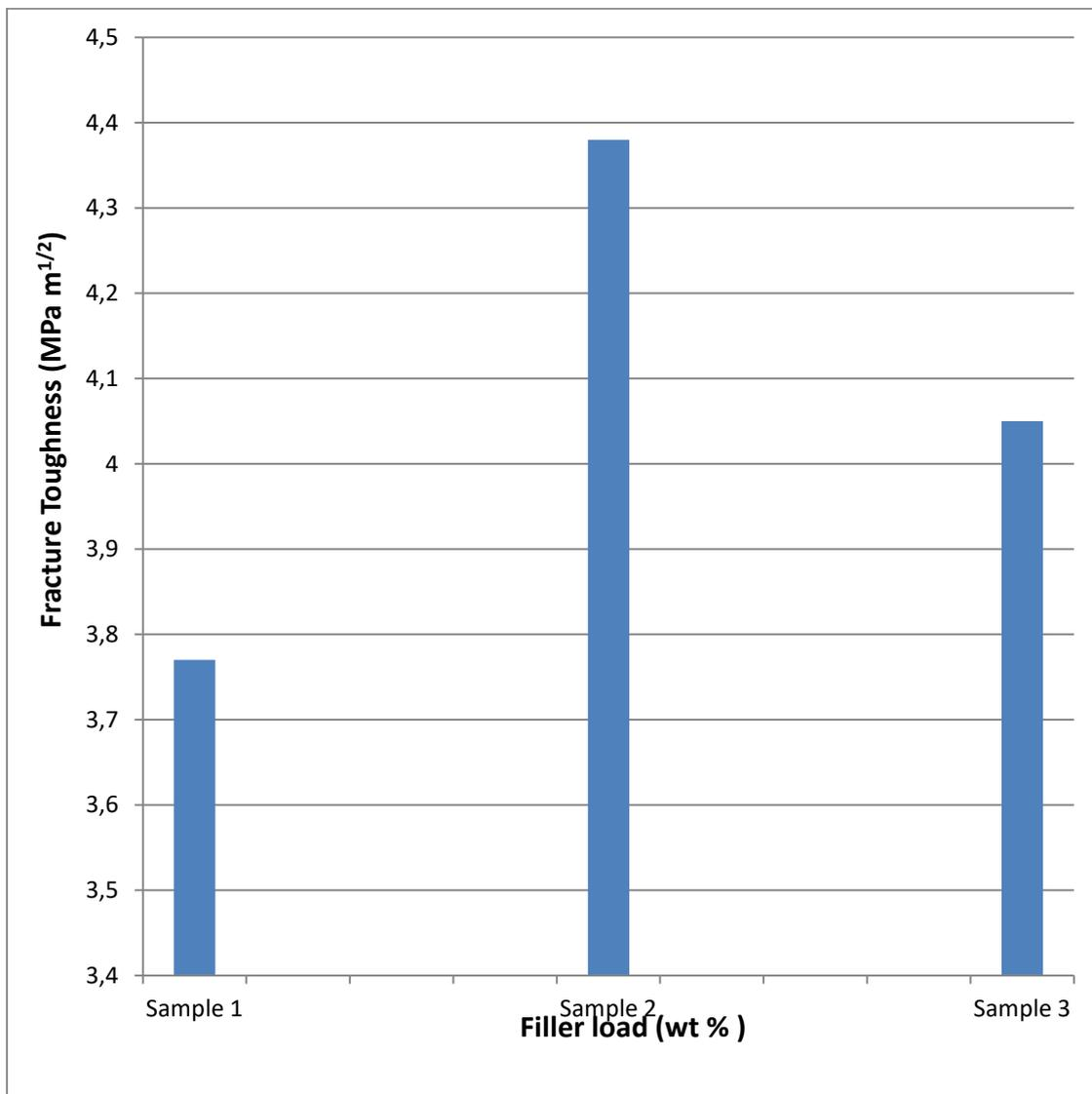
Figure 1. Effect of Fillers Content (wt%) on The Fracture Toughness ( $K_{IC}$ ) of the Epoxy Matrix
