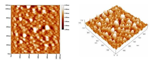
Fig.(5): AFM images for nanostructured film evaporated from S<sub>4</sub> sample, (a) 2D, and (b) 3D.
