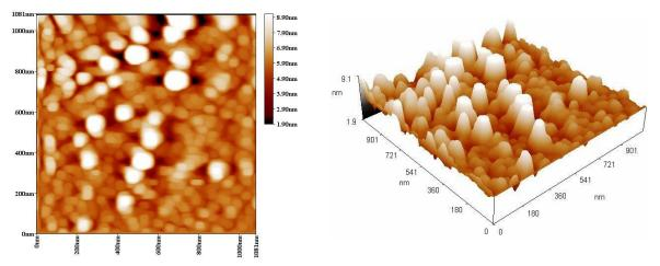
Fig.(3): AFM images for nanostructured film evaporated from S<sub>2</sub> sample, (a) 2D, and (b) 3D.
