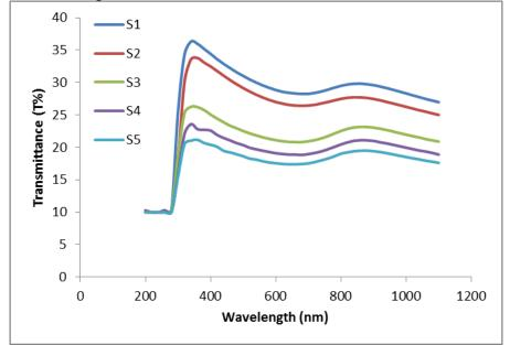
**Fig.(9): Transmittance spectra of Al and Al-Ni-Cr nanofilms measured at thickness of 25 nm.** The measured values of optical energy gap  $E_g^{opt}$  for Al and Al-Ni-Cr nanofilms are listed in Table (3).
