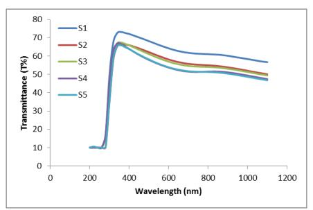
Fig.(8): Transmittance spectra of Al and Al-Ni-Cr nanofilms measured at thickness of 15 nm.
