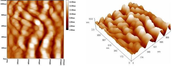
Fig.(6): AFM images for nanostructured film evaporated from S<sub>5</sub> sample, (a) 2D, and (b) 3D
