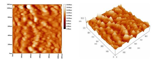
Fig.(2): AFM images for nanostructured film evaporated from S<sub>1</sub> sample, (a) 2D, and (b) 3D.
