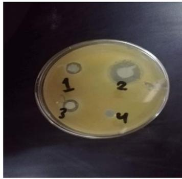
**Fig.(11) Epoxy/ZnO solution by agar well diffusion**
