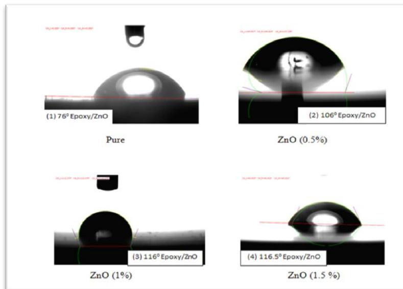
**Fig.(12) Wettability angle of ZnO/ Epoxy composite coating at different ZnO ratios**
