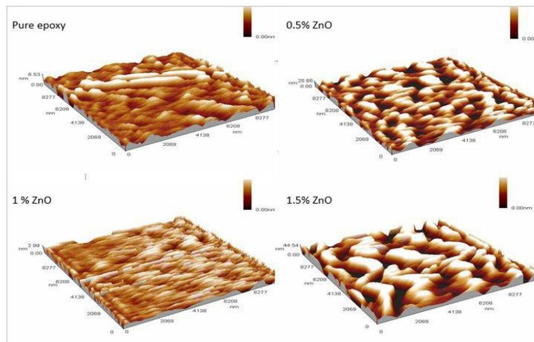
**Fig.(13) AFM image of ZnO/ Epoxy composite coating at different ZnO ratio**
