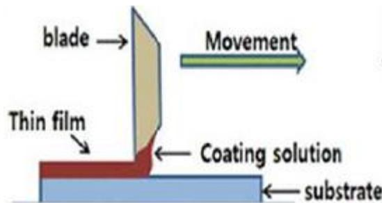
**Fig. (2) Doctor Blade method for coating [15]**
