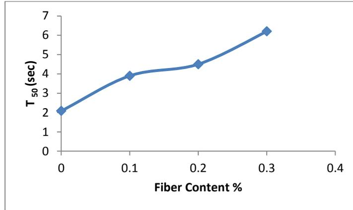
**Fig. (5) Variation of Slump Flow Time T50 (sec) with PF Content %**
