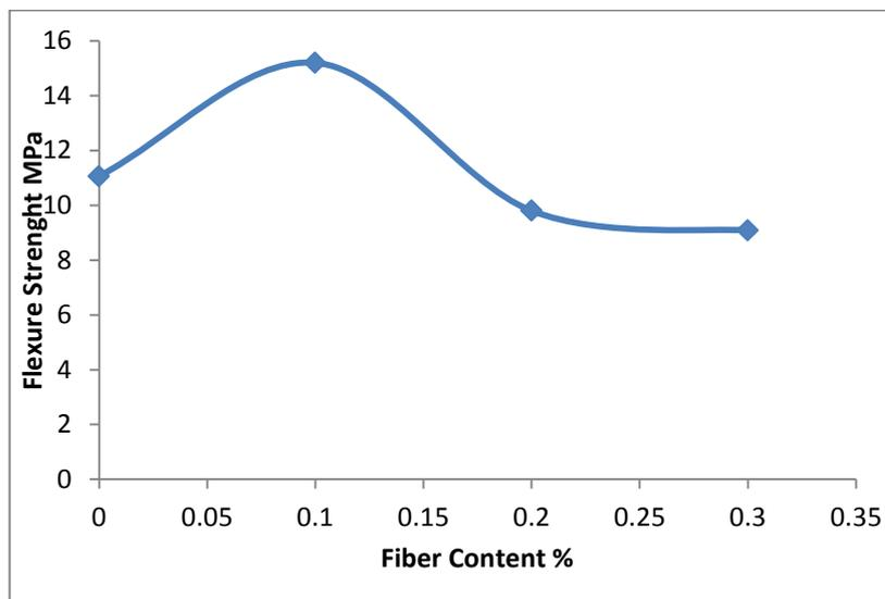
**Fig. (9) Variation of flexural strength with PF Content %**
