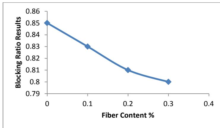
**Fig. (6) Variation of Blocking Ratio Results with PF Content %**
