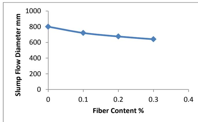
**Fig. (4) Variation of Slump Flow Diameter (mm) with PF Content %**
