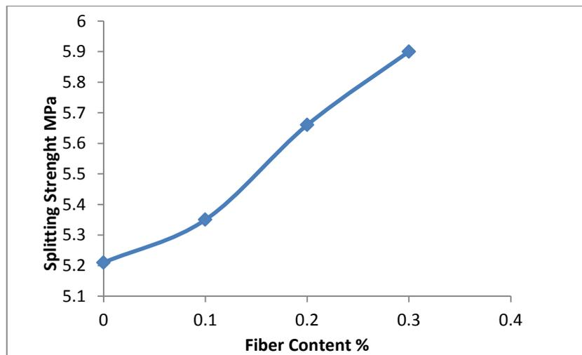
**Fig. (10) Variation of splitting tensile strength with PF Content %**
