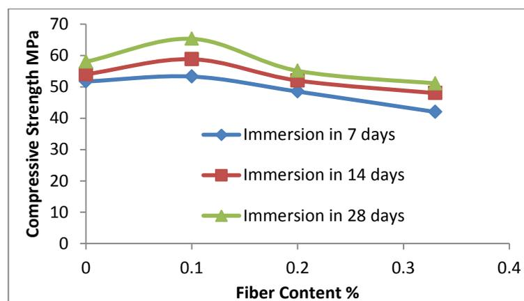
**Fig. (8) Variation of compressive strength with PF Content %**
